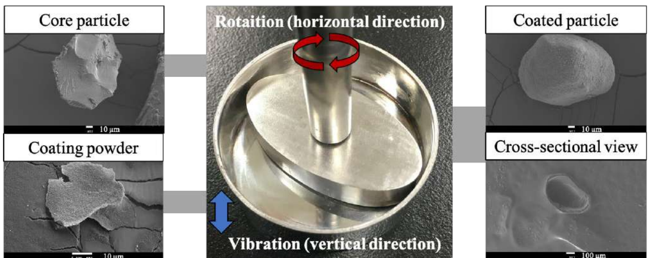
Fig. 1. A schematic diagram of the dry particulate coating system
